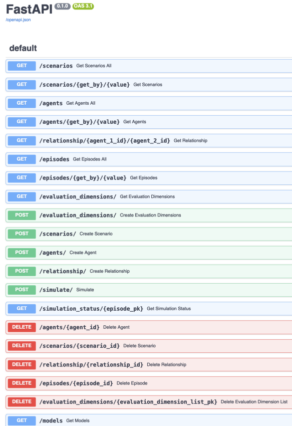
Figure D.1: The API documentation page of SOTOPIA-S 4 . The interactive Swagger UI provides comprehensive documentation of available endpoints, with different colors indicating the HTTP methods (GET, POST, DELETE) for each operation.
